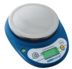
Effortless to transport and store, the CB compact balance offers a streamlined design that is ideal for weighing small quantities in laboratory settings. The backlit display is easily visible from a distance or in less-than-optimal lighting conditions. A sealed keypad, ample stainless steel pan and solid ABS housing make the CB simple to clean. CB balances can be powered with two AA batteries (included) or an optional power adapter, while an auto poweroff feature helps conserve battery life.
